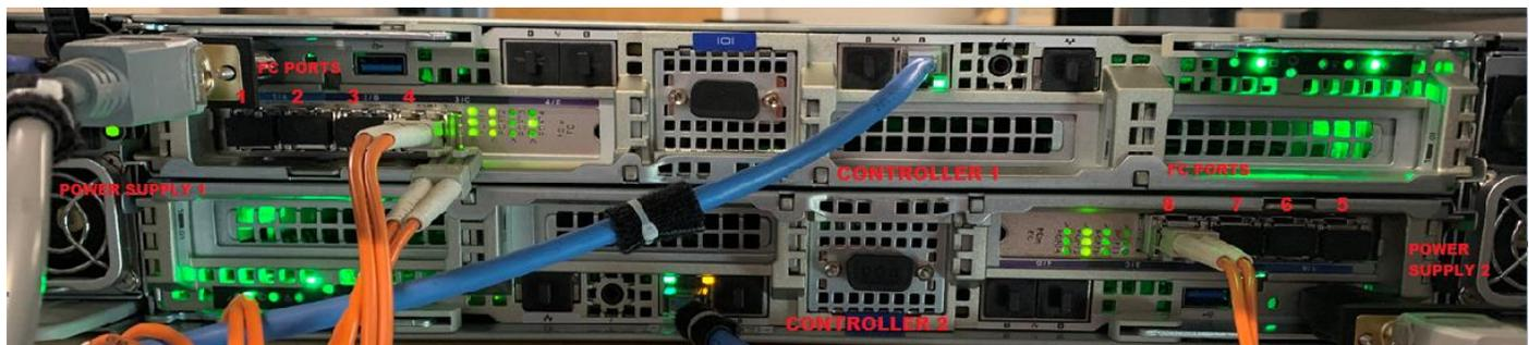
Rear view of QV2020 or 4 port QV1020. QV1020 has option of 2 ports
