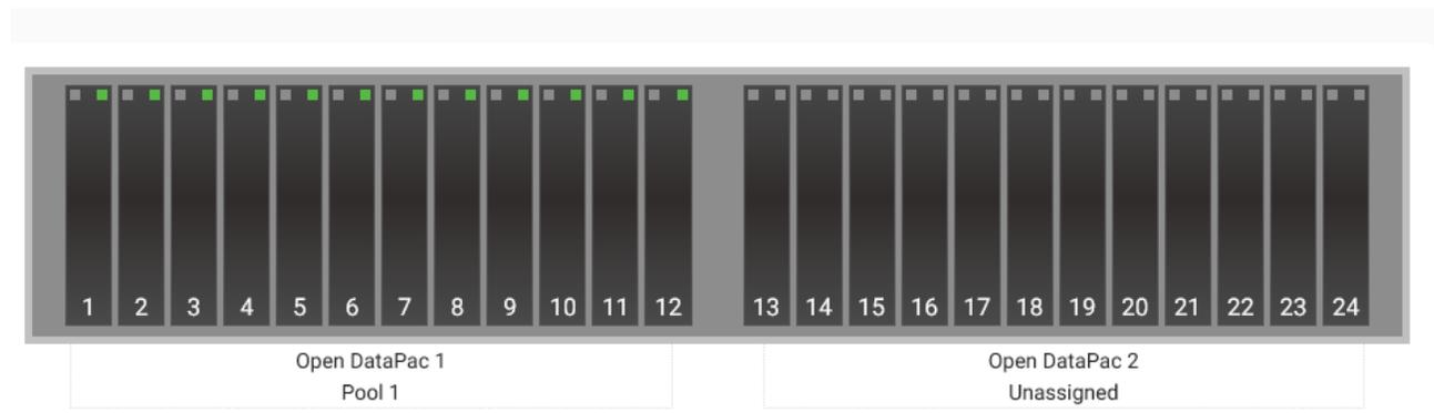
A drive Green LED indicates it is installed and ready for use or in use.
