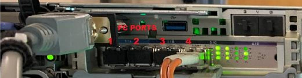
Controller 2 is the bottom controller. FC ports are numbered right to left, as shown below..
